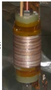
Picture of YBCO coil on winder
