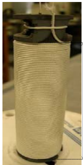
Picture of Bi-2212 coil after heat treatment
