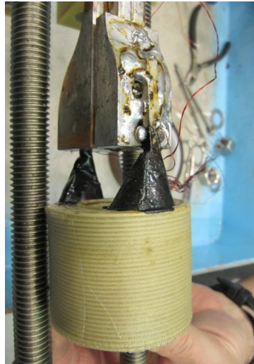
Top: Cross-section of the multifilamentary Bi-2212 wire used in small test coils (bottom) without silver leakage problems.
