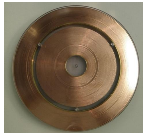
(Top) Winding of sixty-layer model coil. (Bottom) Full scale model pancakes for YBCO coils of the 32T magnet.
